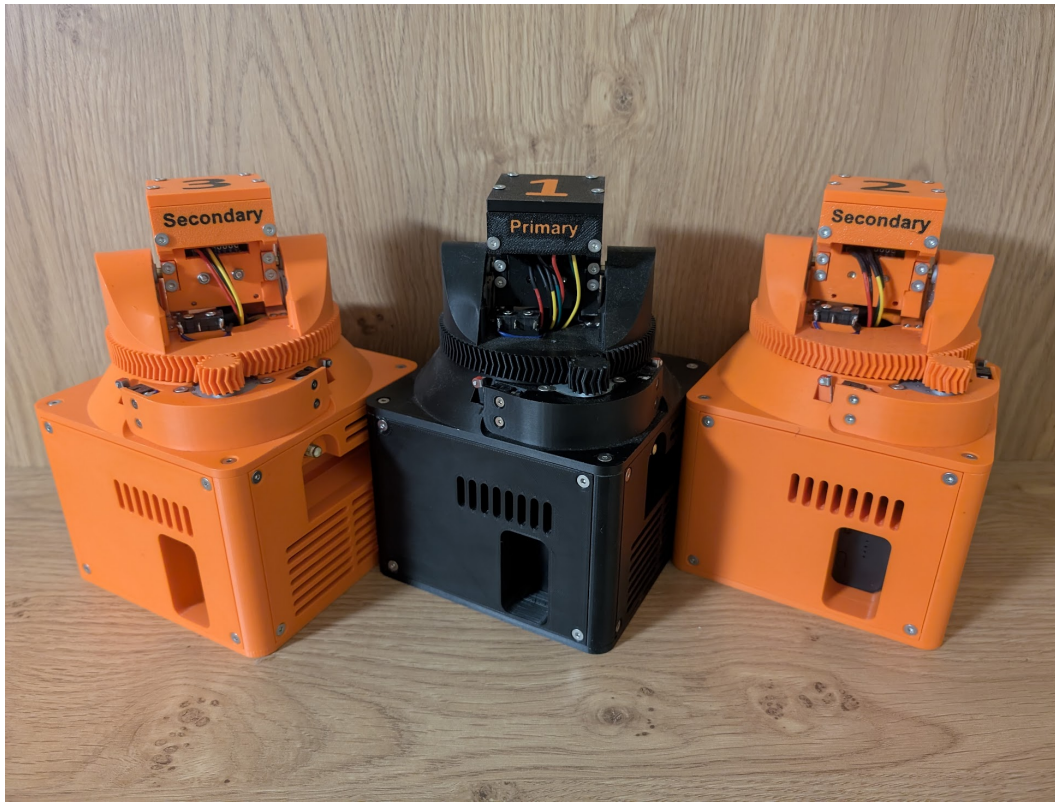
Figure 15: Rear view of all three final stations showing fan outlets and head-mounted components
